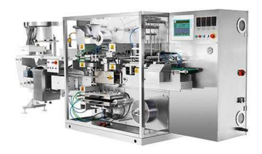
The Alu-Pvc/Alu-Alu blister packing machine of DPPS170A takes full use of compound forming Pvc-Alu (Alu-Alu) foil as packing material to punch beautiful blisters through special punching module. After feeding, detecting, sealing, batch number printing, slitting and punching, the product made by the machine presents a fine appearance and reliable condition.
