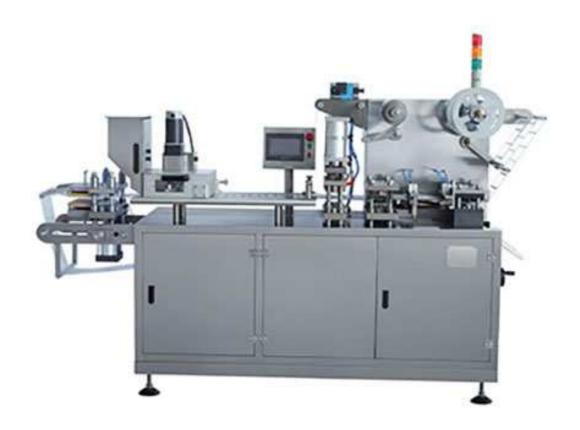
The product is specially designed for hospital dosage room, laboratory institute, health care product, middle-small pharmacy factory, and featured by compact machine body, easy operation, multi-function, stroke adjustable, long durability etc, it is suitable for the Alu-PVC package of medicine, food, electric parts etc. Aided forming Pre-cutting Inspection and rejecting control systems. Print mark registration Automatic feeder.
