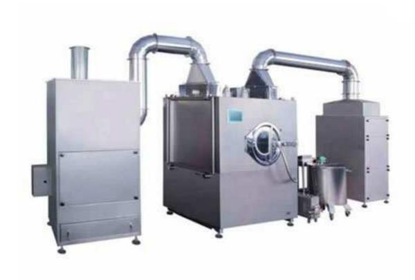
The machine is a kind of mechanically and electrically integrated coating equipment with high efficiency, energy conservation, good safety and good cleanliness for organic film coating, water soluble coating, dripping pill coating, chocolate and candy coating of tablets, pills and candies.
