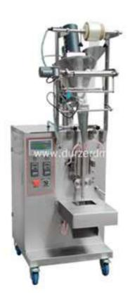
Automatic Sachets Packing Machine is suitable for three side sealing and four side sealing packaging of powder materials. Equipped with Powder Auger Elevator or Pneumatic Vacuum Feeder. It can realize automatic measurement, bag making, filling, sealing, cutting, continuou making sachet and finished product conveying. You can also add optional features, such as easy tearing, printing Labelling Machine.
