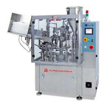
PLC control unit, servo motor controlled film transport, connection apparatus and hoses for aspirator group. Metallic grey colored and surfaces of the machine that are in contact with the product made stainless
