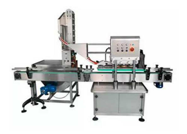
This versatile in-line capper handles a wide range of containers at speed to 200 bpm and offers a quick and easy change over routine that maximizes production flexibility.
