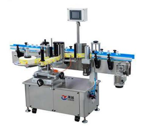
This automatic labeling machine is suitable for cylinder like bottles or cans. It is suitable for single side and double side labeling, the distance between front and back side label stickers is adjustable. This machine can be equipped with circumferential positioning detection device which helps to achieve to specific position labeling. It can be also equipped with the date coder for printing production date and number, if you need these please contact us.
