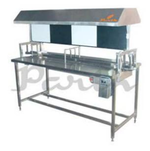
Inspection table is equipment consisting of a three-track conveyor with a hood with lighting arrangement and visual inspection background of alternate black & white color. Inspection table (Inspection Conveyor) have stainless steel structure with moving S.S. slat chain. Structure made out of S. S. square pipe & supported on adjustable bolts.
