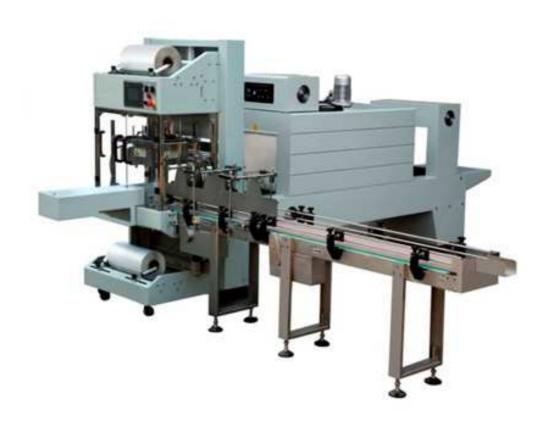
The automatic bottle shrink wrapping machine is up and down power proximity switch control, effectively prevent the mistake cutting., at the same time to ensure the safety of operation person. High-performance, omron PLC for the whole machine is stable, reliable operation, and has played a key role.
