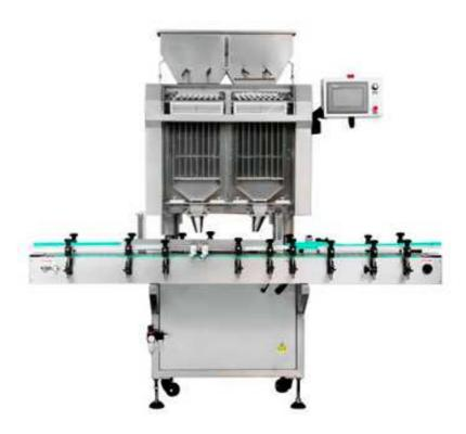
Electronic soft gel counting machine, is manufactured with high-response PLC and advanced European and American laser induction technology. Exquisite appearance, beautiful appearance, convenient maintenance. Widely used in the pharmaceutical, health care, food, pesticide, chemical and other industries. Pill counting machine can be used as a stand-alone machine. It can form a complete bottling production line with other bottling equipment produced by our company.
