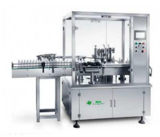
The rotary stopping machine is suitable for stopping of bottles with inner stopples in such industries as medicine, daily chemical industry, biological industry or other industries. It adopts continuous bottle moving mode and mechanical hand vacuum stopple grabbing and stopping. It can work with various packaging machines for integrated production.
