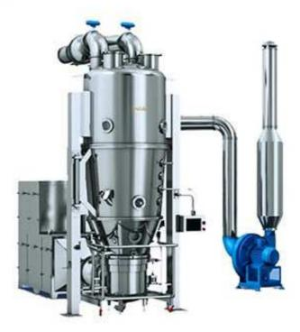
The machine is a process machine widely applied for solid preparation production in the pharmaceutical industry. It has such functions as mixing, drying, granulation functions etc. It is also widely used in such industries as medicine, chemical, food, etc
