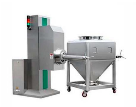
LDTH series bin blender is widely applied in pharmaceutical production to mix dry powders with dry powders or granules of different substances. This machine can be equipped with multiple models of hopper and applied in large or medium enterprises. The single machine can mix medicine of different substances and batches according to technical requirements so that it can be multifunctional.
