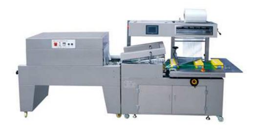
Type: L-type fully enclosed, Fully automatic shrink wrapping machine, Automatic Shrink Machine, BMD-450C automatic shrinking machine, automatic shrink wrap machine.
