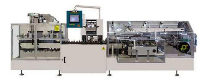
GHD-220 Multi-function Cartoning Machine is made of series of precision gear and device, all the work like drawing carton, opening carton, drawing specification, wrappage filling, batch number print and carton closing can be finished one time, completely in conformity with GMP.
