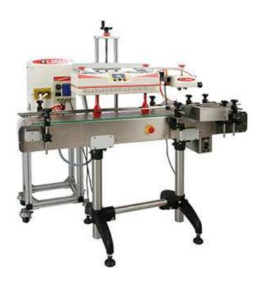
Induction Aluminum Foil Sealing Machine is used for PP, PE, PET, PS, ABS, HDPE, LDPE and glass bottles, which utilizes electromagnetic principle to produce instant high heat to melt aluminum foil that then adheres to the opening of the bottles, reaching the aim of wet-proof, leakage-proof, mildew-proof and extending preservation time.
