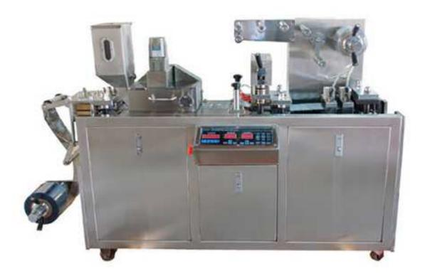
This machine can continually and automatically complete the packing proceedings, is blister cap form-taking, medicine-feeding, heat sealing, printing lot no, and cutting into format. It has advantage as compact structure, full function, gear wheel working, and accurate Synchronization, stable cooperation, easy to replace the mould, low cost and needn't to equip Auxiliary unit. Turn on power and connect it with cooling water, you can produce in a large scale.
