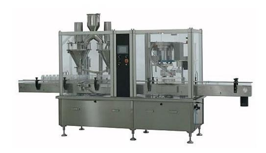
This GSF30/2 automatic powder filler combines the functions of filling and capping. Thus, it wins broad application to packing milk powder, monosodium glutamate, solid beverage, dextrose, coffee, solid drug, etc.
