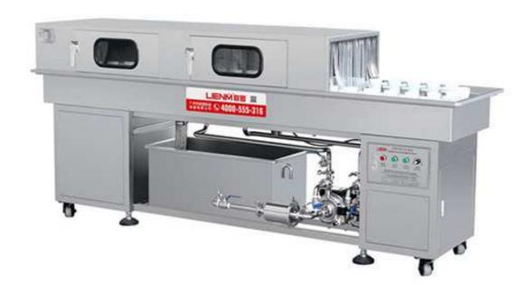
Guangzhou Manufacture Double Line Bottle Washing Machine Positive up and down the bottles, intermittent flushing of the positioning, to ensure accurate high-pressure jet of water sprayed into the bottle and, with two water separator, circulating water tank, water pump, a tap water rinse, a pure water rinse, effect of variable frequency speed control, water control.
