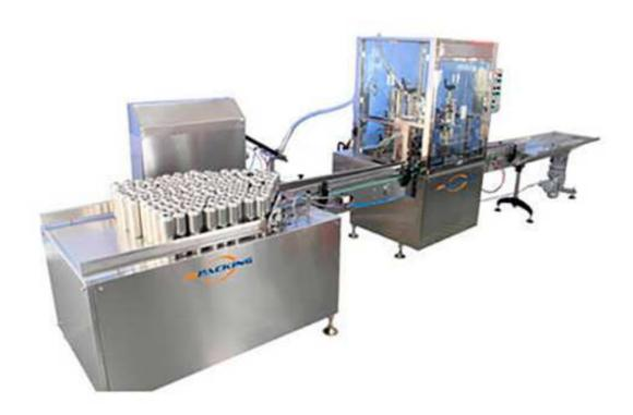
2800A aerosol filling machines is a small automatic aerosol filling assembly line, CE approved. It design two sets liquid filling machine, valve correct, sealing machine and two sets gas filling in a rotary table.
