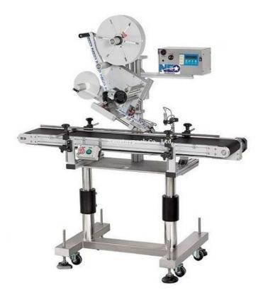
Top Tamp Labeling Machine NLS-450 is designed for particular shape of bottles which can't stand stably and hollow or rough surface.
