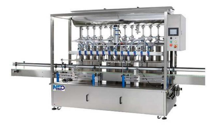
NFP-4127 Automatic 12 Heads liquid Filling Machine works well with any free flowing liquid or thick products like shampoo or paste. Controlled by PLC and HMI control system for ease of operation. With tool-free disassembling design and customized filling nozzle, it can surely boost the production and efficiency.
