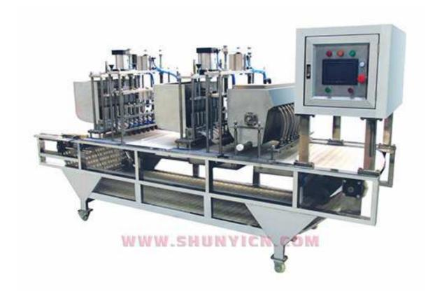
The CD serials filling and sealing machine is suitable for the filling before baking of the thick sauce product such as cake, egg tart, oblate. The machine can fill the multiple containers in the tray at the same time; it also can fill the single-row appointed container. The machine adopts PLC control system and made of all stainless steel, meets the requirements of the food industry, easily operation. The machine is the ideal filling device for the baking food.
