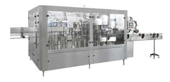
The series equipment is used in hot filling and sealing of tea, fruit juice drink and etc. The machine integrates washing, filling and capping together. It is good equipment for hot filling with scientific and reasonable design and easy operation.
