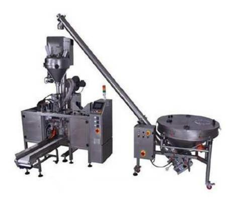
This machine is specially designed for packaging all kinds of powder, such as coffee powder, milk powder, curry powder, protein powder, pepper powder, etc., into premade pouches such as flat pouch, gusset pouch, stand up pouch, zipper pouch, doypack, etc.
