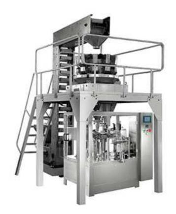
Vertical Stand Up Zipper Pouch Doypack Rotary Packing Machine with Multihead Weigher can be suitable for automatic packing for grain and solid food, such as beans, nuts, dry fruits, candy, cereal, chocolate, biscuit, peanut, capsule, seeds, chemicals, sugar, etc. Different kinds of product with stand up pouches, doypack with zipper, 3 side seal bags, 4 side seal bags, flat bags, pouch with hole, spout pouch, etc.
