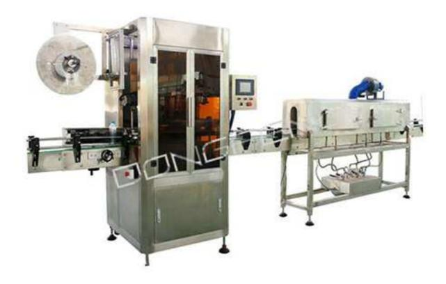
The sleeve labeling machines is the labeler for PET bottle and sleeve label by shrink label principle.
