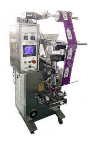
The tea powder packing machine is suitable for pouch packaging of non-flowable powdered materials. The production materials are all made of stainless steel, and the contact parts with the materials are made of 304 stainless steel, which fully meets the food hygiene standards.
