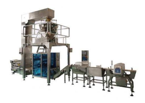
Vertical Automatic Weighing and Packing Machine is equipped with Z Conveyer to coordinate with Multihead Weigher. Suitable for packaging many different kinds of products; such as puffy food, candy, shrimp roll, peanut, popcorn, cornmeal, dried fruit, seed and sugar etc, which shape is roll, slice and granule.
