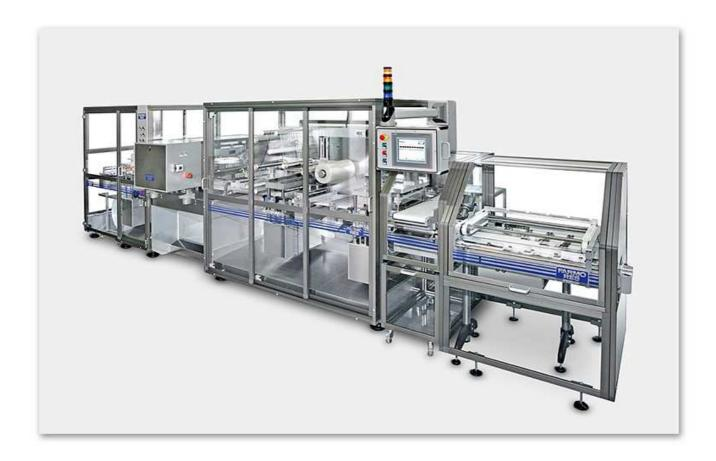
Prima K7 is the new automatic thermoforming machine with a balcony constructed frame and driven by servo motors for packing syringes vials and ampoules in laminated plastic materials. Technical innovations: compact frame, automatic positioning of sealing, perforation and cutting station, operator side reel loading, fast adjustment of the forming clamps, improved design so using less space in the loading area.
