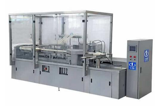
Installation AGF used for filling and sealing the glass vials of glass of 1 ml - 20 ml, it will automatically perform the following procedure: feeding the packaging, filling with nitrogen, filled with liquid drugs, heating, sealing of, the final product unloading. The equipment can be used both independently and in conjunction with the installation of an ultrasonic washing and drying-sterilizer.
