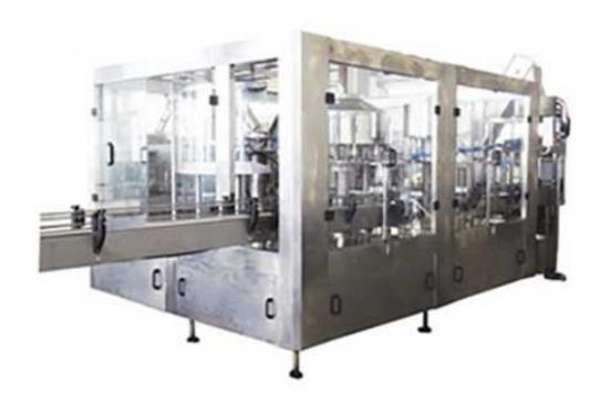
3L-10L water filling machine can be classified into atmospheric pressure filling machine and isobaric pressure filling machine. It depends on the production that customers want to produce. Generally mineral water production line, and pure water production line will choose atmospheric pressure filling machine. Carbonated drink production line, oil production line and fruit juice, fruit tea production line will choose isobaric pressure filling machine.
