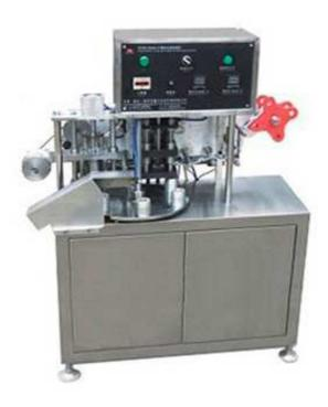
The machine apply to 5 Gallon cap labeling and sealing, it's suitable for 5gallon cap manufacture and water factory.
