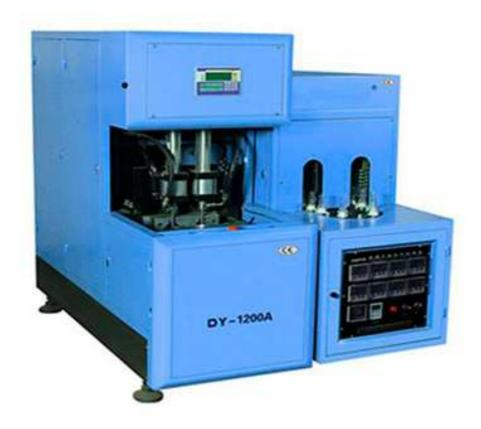
DY-1200A semi-automatic bottle blow molding machine is suitable for producing PET plastic containers and bottles 10-2000ml.
