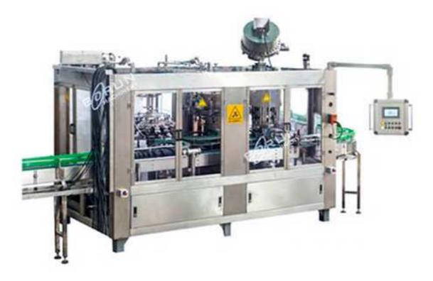
This machine combines automatic rinsing, filling and capping in one machine, it's specially designed for beer glass bottle with crown caps. The machine has the feature of compact structure, low noise, easy maintenance and operation. And it adopts two times vacuuming to minimize the oxygen level during beer filling.
