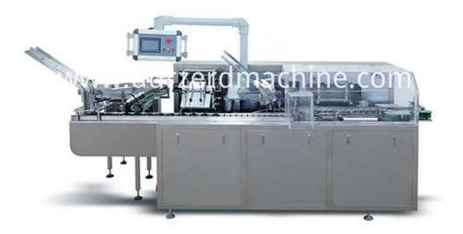
This small Carton Box Packing Machine is suitable sachets into carton. It can fold leaflets, open cartons, insert the products and leaflets into cartons, emboss, tuck-in or hot-melt closures and automatically discharge cartons. It can also be connected to Sachets Packing Machine or Bottle Filling Machine to form a complete production line.
