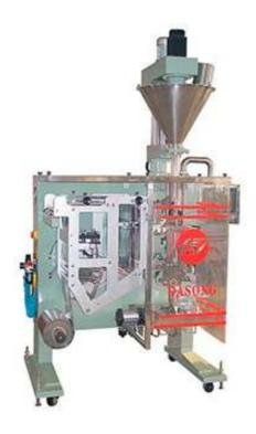
The 1kg powder packing machine is widely used to pack any powder in a back sealed bag. The process of measuring, bag making, filling, sealing, printing and cutting can be done automatically
