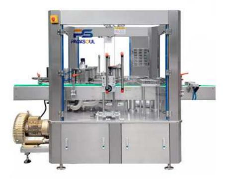
PACKSOUL PSL series automatic labelling machine is specially for attaching opp and bopp labels to round and cylindrical containers of water, beverage, wet tissue and daily chemical product.
