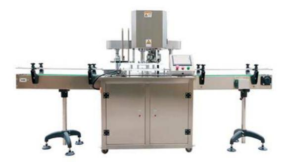
The automatic can sealing machine is suitable for sealing various various tin cans, aluminum alloy cans, paper cans, etc.
