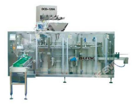
This machine suitable for prefabricate flat bag, doypack filling and sealing. Controlled by PLC program, can used for filling granule, clump, powder, pasty, liquid and other material. This machine can take and open the bag, filling and sealing automatically. High degree of automation, operation simply and convenient, measured accurately, the packing effect smooth and beauty. It is the ideal packing machine for food, grain, seed, chemical, daily chemical and pharmacy industry.
