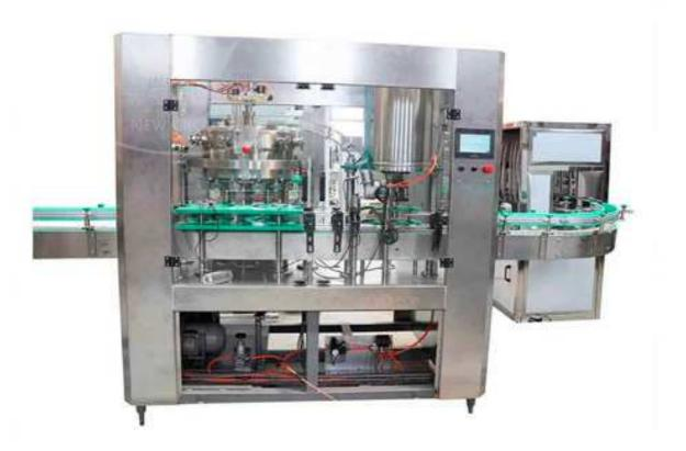
Our newly designed DCGF serious monoblack CSD filling machine is designed for aluminum can and metal tin can filling, it can suit for can size between 150ml to 750ml, can customized to maximum of 1000ml. On machine surface is only leaving 3 points of bearing support point which makes drainage so easy and without any dirt stain.
