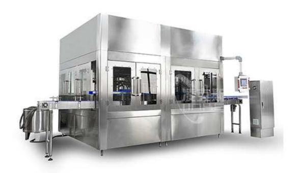
This machine is mainly used for washing, filling, capping non-carbonated drinks such as pure/mineral water. The machine shorten the contact time of the drinks material and outside, increasing the sanitation condition productivity and economy benefit.
