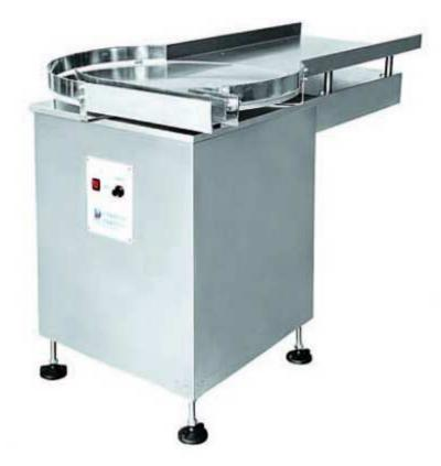
Fully automatic bottle unscrambling machine, max speed is 120 bottle/min
