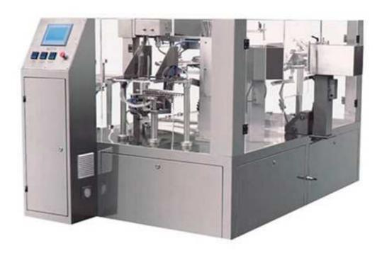
This machine is a full-automatic packaging machine, which integrates machine, light, electricity and gas. It has a wide range of packaging and is suitable for solids, liquids, sauces, powders, granules, pickles, irregular materials, etc. For materials, simply select different metering and filling devices according to different materials.
