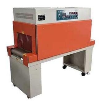
The heat shrink packaging machine can reduce the possibility of the product being dismantled and stolen. When the shrink film shrinks, it produces a certain tension, so it can wrap a group of items to be packed tightly and play the role of strapping. Especially suitable for the collection of multiple items and pallet packaging.
