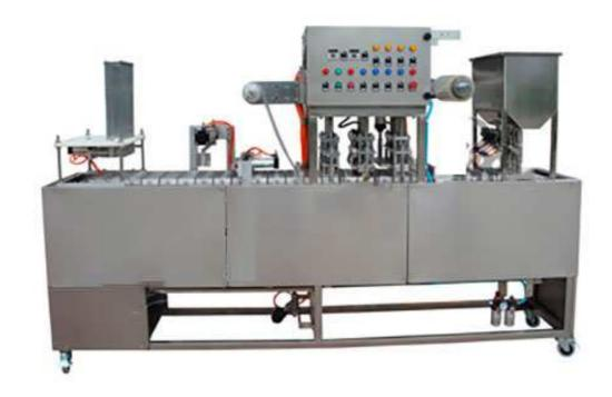
GF-4 Cup washing and sealing machine for a variety of mineral water, beverages and other products. The machine adopts Japan OMRON programmable logic controller, pneumatic control components, intelligent digital temperature control system, stainless steel, with automatic washing cups, sealing high strength, good sealing, low failure rate and other characteristics. It is the preferred product to choose of the enterprise automation production.
