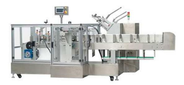
The cartoner machine automatically picks the carton and forms the carton, the worker manually puts the products on the moving conveyor, and when it's moving to the formed carton, the machine pushes it into the carton, sealing the carton. If you want to save the labor cost, you can add a robot to place the goods on a conveyor instead of one person.
