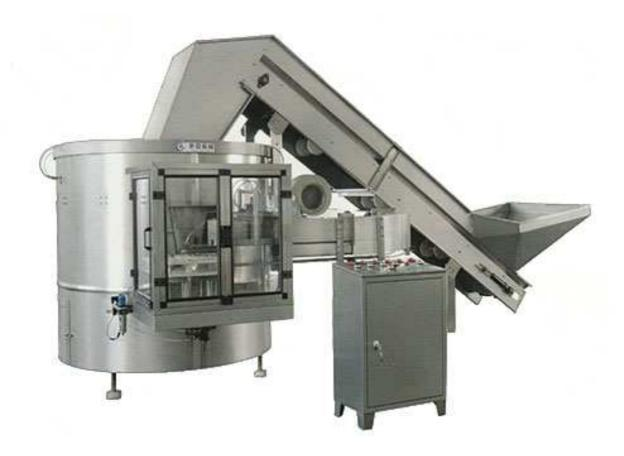
UPS Automatic High Speed Bottle Unscrambler Series is used for arranging Plastic bottles in an orderly on High Speed by Neck Hanging system thru an Air Conveyor into the 3 IN 1 Monoblok filling machine. With production capacity ranging from 6000 bottles to 20000 bottles an hour.
