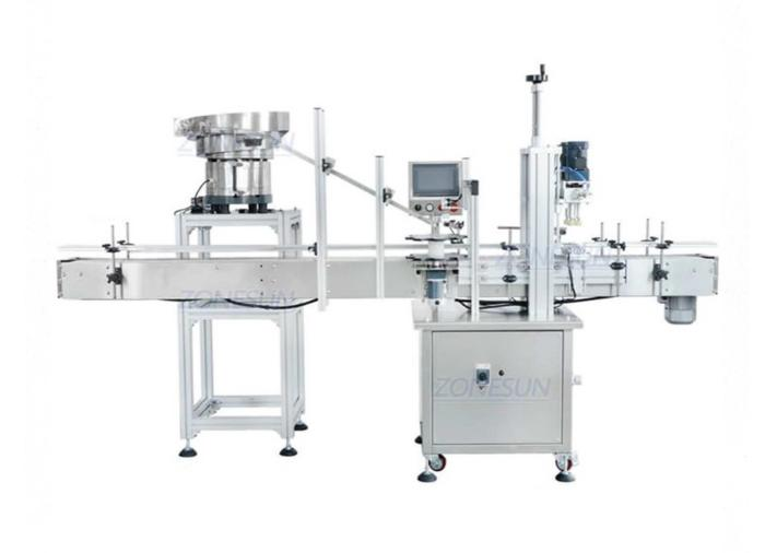
This full automatic capping machine is equipped with a cap feeder, which can orient bottle caps. Typically, the cap feeder can be customized by making adjustments to the bowl for different sizes of caps. Larger caps and higher speeds may require larger bowls. These two machine can achieve automatically feeding caps and cap bottles, save labor and reduce production error.
