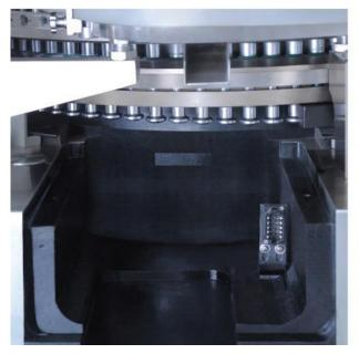
Module design, which is easy to assembly and disassembly the punches&die.
